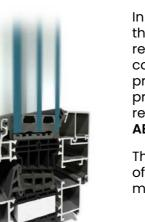
In terms of technical properties the MB-86US system meet all requirements concerning energy conservation and environmental protection. The structure of the profile similarly to basic MB-86 system has three variants depending on requirements of thermal insularity: MB-86US ST, MB-86US SI and MB-86US AERO with the use of modern insulation from aerogel.
