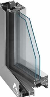
The MB-79N is a state-of-the art and economical addition to the Aluprof window & door systems. It has been designed to outperform typical thermal insulation requirements. The MB-79N series can be used to fabricate fixed, side-hung, hopper, tilt-and-turn, and hopper-and-slide windows, as well as single and double exterior doors, and storefront solutions complete with doors.
