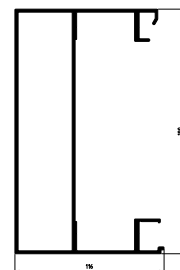
Edge purlin with dimensions of 120×190 mm
